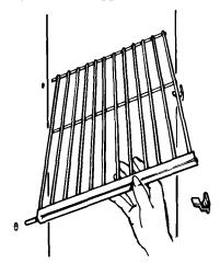
2. Pull shelf sideways until rods come out of **holes** on left wall.
